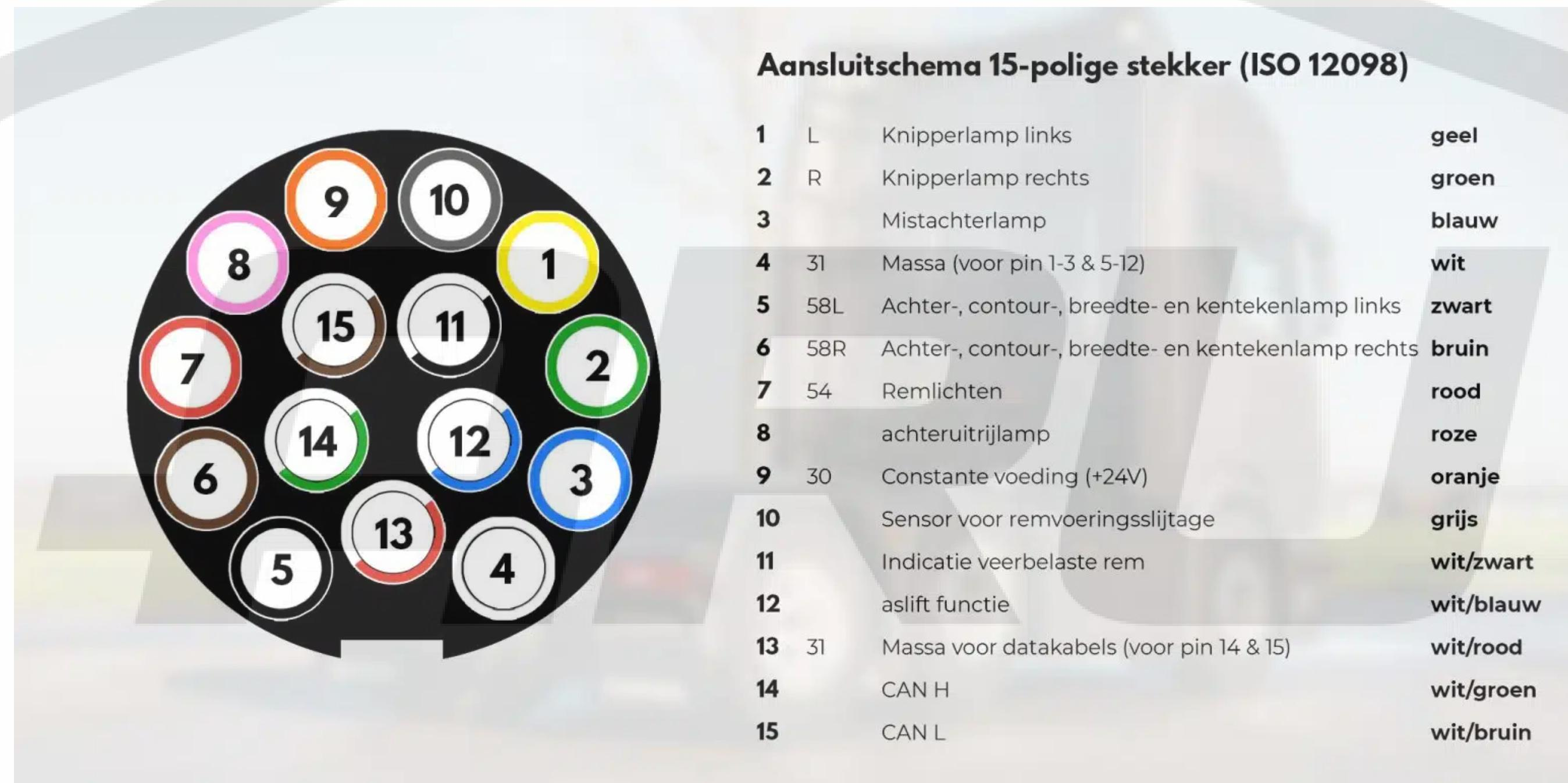
This diagram illustrates the standard 15-pin electrical connection (ISO 12098) between a towing vehicle and a semi-trailer. It defines the pin numbering, assigned lighting or auxiliary functions, and conventional wire colour codes for the 24 V system. The ISO 12098 standard ensures compatibility of electrical circuits for braking, lighting, and communication between vehicles and trailers.
